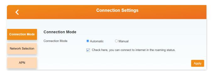
To enable the hotspot to connect to the internet automatically after it is powered on, select Automatic, and click Apply.
