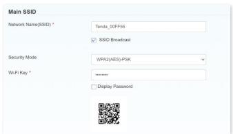
Step 5 Scan the QR code using the Wi-Fi scan function of your mobile phone to connect to the wireless network of the hotspot;
