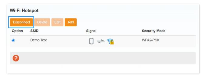
After the SSID is disconnected, you are allowed to delete the SSID from the list.
